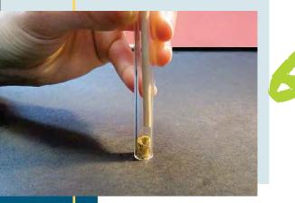
Insert screens into the stem. Place the stem on prep work space and push the screens down with a wooden stick so they are tightly packed.
